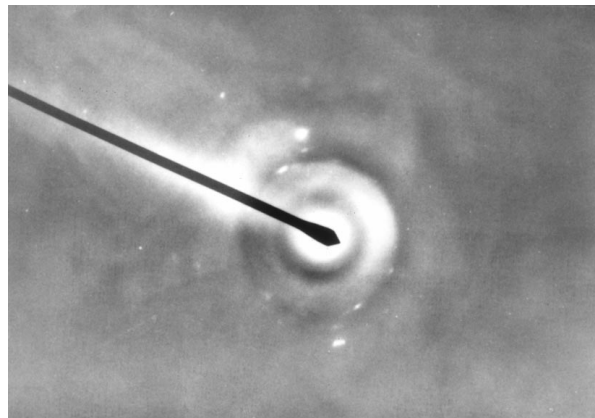
Figure 2 Transmission electron diffraction pattern from repeatedly rubbed zirconia ( 3 \times 10^4 traversals).
